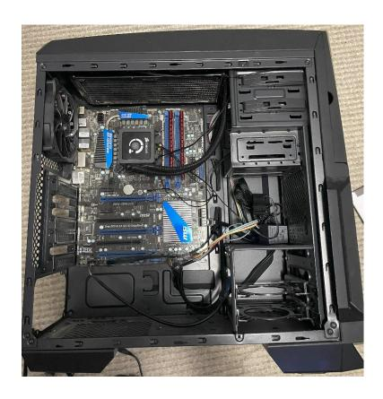
From here, all I need to install is the GPU and power supply. Luckily, this saved a lot of time and money due to the fact that I did not need to build a system from scratch. The finished build can be seen in the pictures below.
